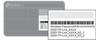
The default wireless network names (SSIDs) and password are printed on the label at the bottom of the router.
