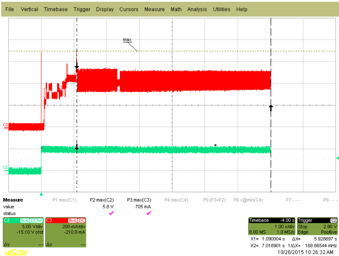
Figure 1. 8TB and 6TB Typical 5V startup and operation current profile
